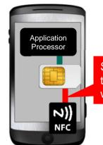
SIM-NFC connection through a single, wired interface
